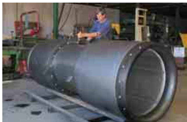
An additional fan for the M5 East Tunnel.
