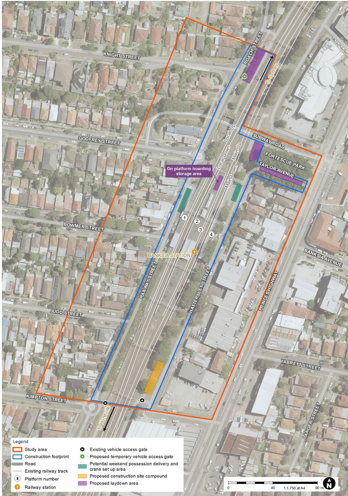
Figure 2: Banksia Station – site location and locations of temporary site facilities and laydown areas
