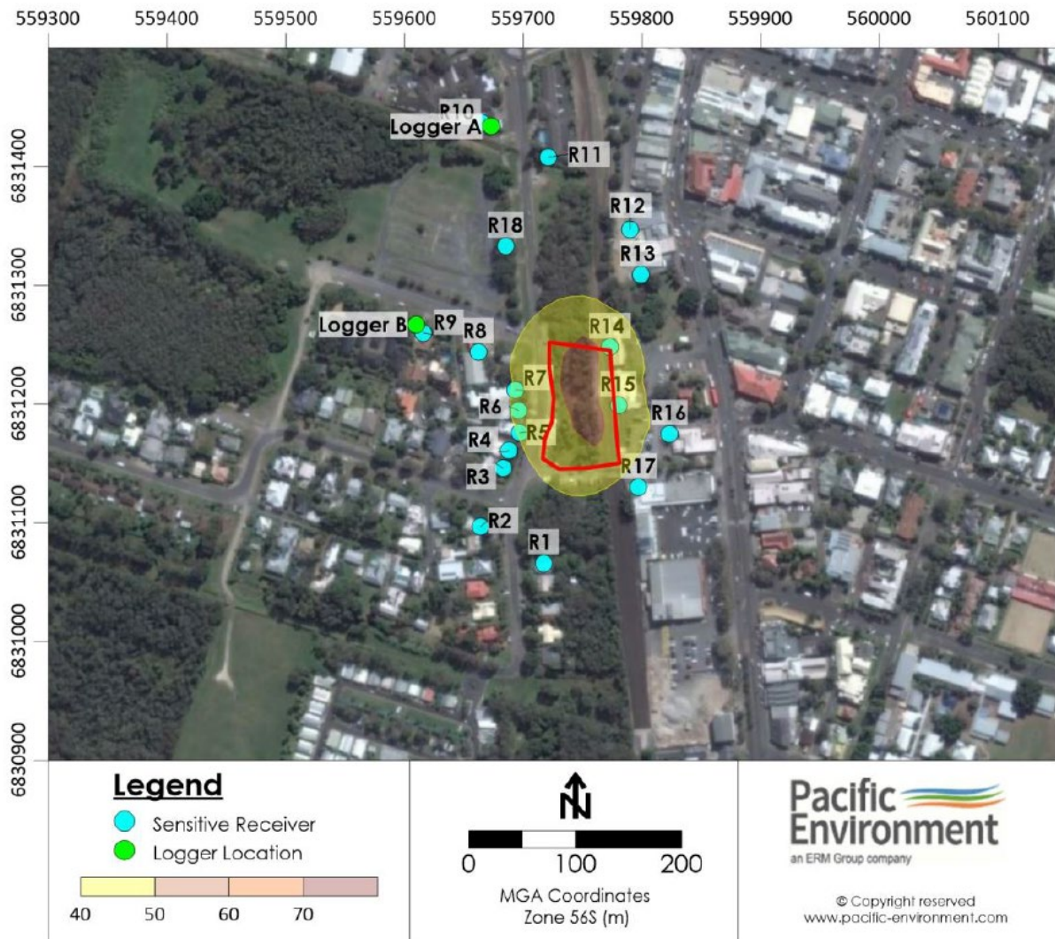
Figure 5-10: Noise contours - average vehicle movements at the proposal operational footprint (night time)
