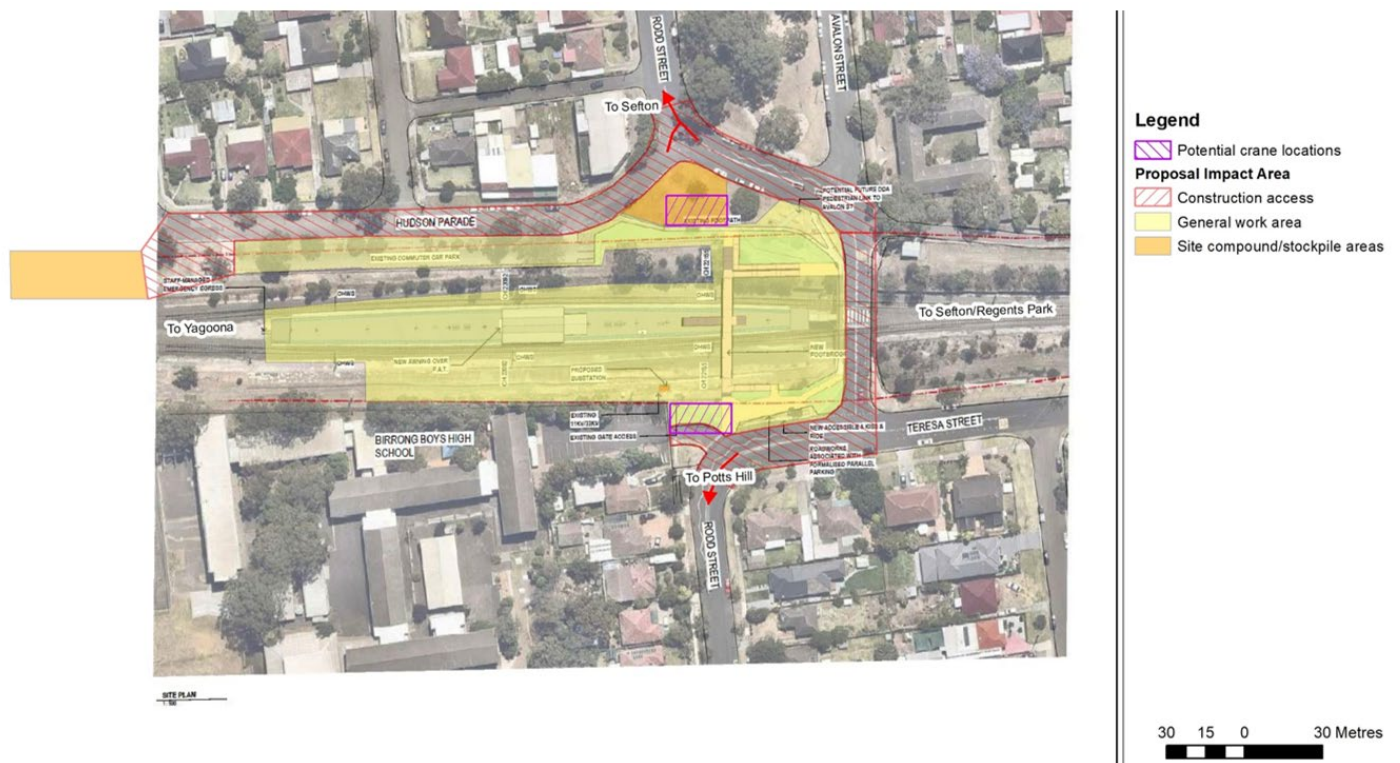
Figure 10 Temporary laydown, storage and amenities areas
