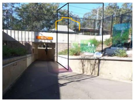
Figure 36. View east from the Wongala Crescent entry to the station towards the site of the proposed lift from the subway to the platform. The location of the western lift structure (black outline in right foreground) would largely obscure all views of the lift structure for the platform behind it (approximate location and profile shown in yellow).
