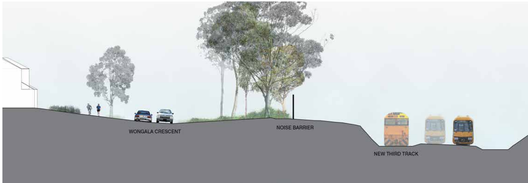
Figure 3-22 Typical cross section view
