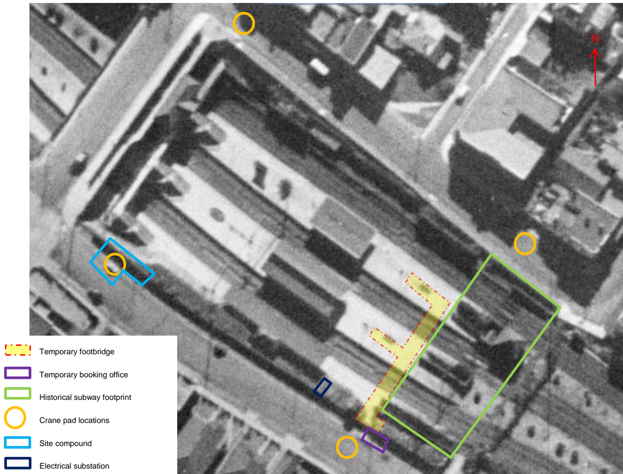
Figure 9 Overlay of approximate location of proposed temporary works on 1943 aerial. (Source: NSW Property and Information)
